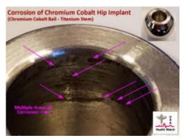
Picture of a Hip Implant showing multiple areas of chromium cobalt corrosion. Corrosion such as this can be associated with elevated cobalt levels and encephalopathy. Click on the picture to enlarge.
